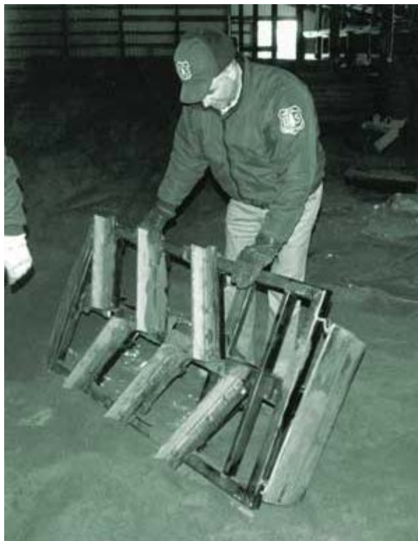
Figure 27—Dick Dufourd inspect "Big Bertha." It's aggressive cutting action and weight are too much for an ATV to handle, but it works great in sandy soil when towed by a tractor.
