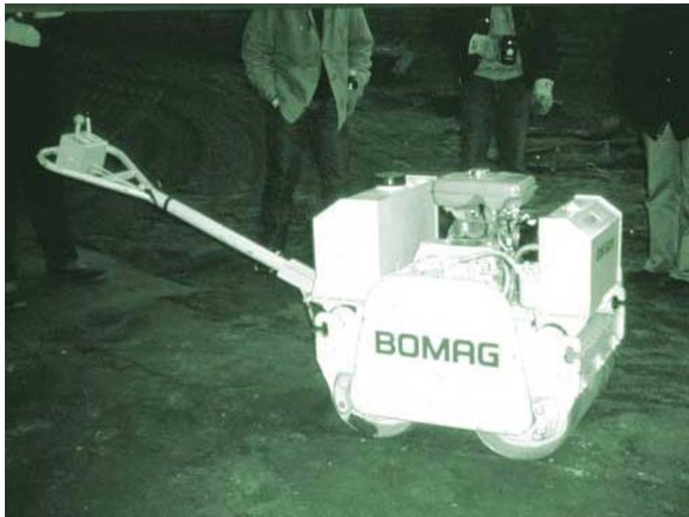
Figure 28—This Bomag walk-behind vibratory roller provides excellent compaction but is slow.
