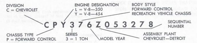
A vehicle identification number is stamped on a combination vehicle identification number and rating plate located on the dash and toe panel.
